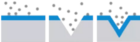
■ Protective Layer ● Oxygen ■ Stainless Steel
